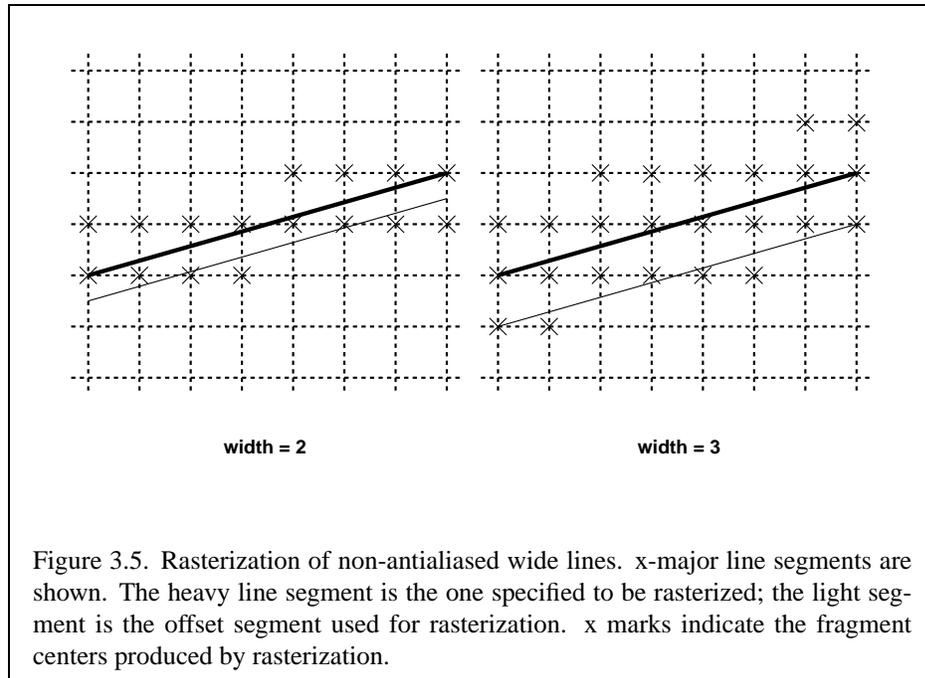
Figure 3.5. Rasterization of non-antialiased wide lines. x-major line segments are shown. The heavy line segment is the one specified to be rasterized; the light segment is the offset segment used for rasterization. x marks indicate the fragment centers produced by rasterization.
