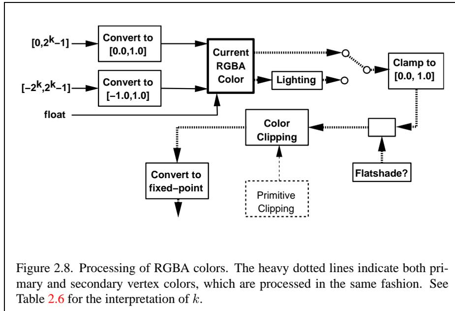
Figure 2.8. Processing of RGBA colors. The heavy dotted lines indicate both primary and secondary vertex colors, which are processed in the same fashion. See Table 2.6 for the interpretation of  $k$ .
