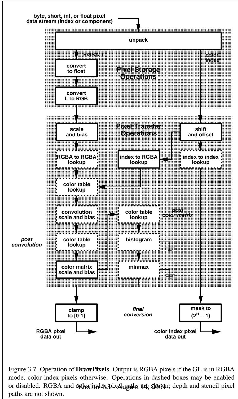
Figure 3.7. Operation of **DrawPixels**. Output is RGBA pixels if the GL is in RGBA mode, color index pixels otherwise. Operations in dashed boxes may be enabled or disabled. RGBA and color index pixel paths are shown; depth and stencil pixel paths are not shown.
