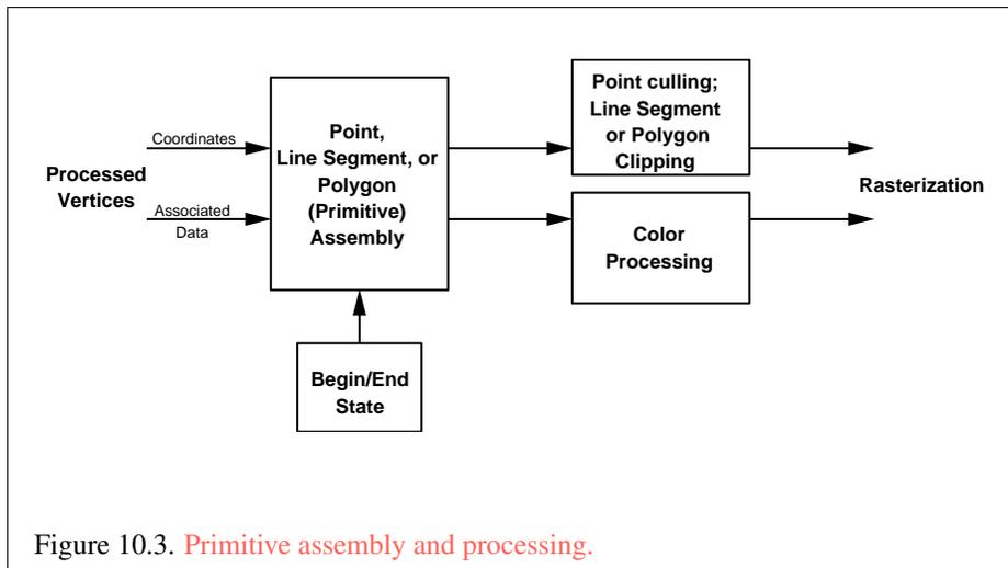
vertex processing. The vertices defining a primitive to be rasterized have vertex coordinates, texture coordinates and colors associated with them. After a primitive is formed, clipping may alter all these attributes.
