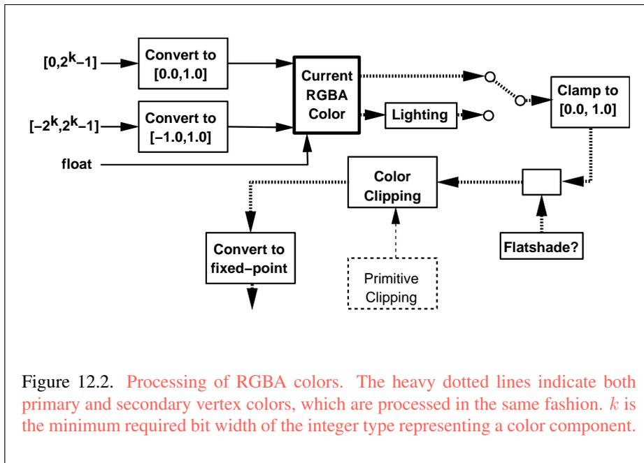
Figure 12.2. Processing of RGBA colors. The heavy dotted lines indicate both primary and secondary vertex colors, which are processed in the same fashion.  $k$  is the minimum required bit width of the integer type representing a color component.
