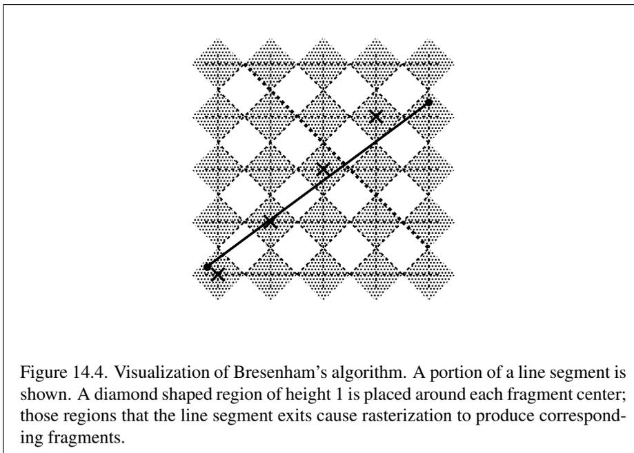
segment starting at  $\mathbf{p}_a$  and ending at  $\mathbf{p}_b$  produces those fragments  $f$  for which the segment starting at  $\mathbf{p}'_a$  and ending on  $\mathbf{p}'_b$  intersects  $R_f$ , except if  $\mathbf{p}'_b$  is contained in  $R_f$ .  $\epsilon$  is chosen to be so small that rasterizing the line segment produces the same fragments when  $\delta$  is substituted for  $\epsilon$  for any  $0 < \delta \leq \epsilon$ .
