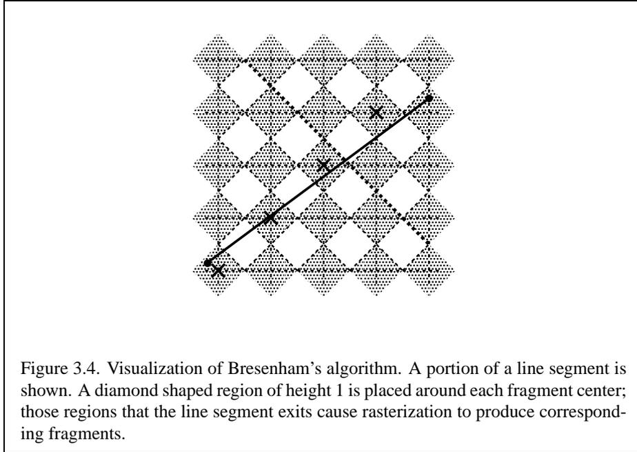
Figure 3.4. Visualization of Bresenham's algorithm. A portion of a line segment is shown. A diamond shaped region of height 1 is placed around each fragment center; those regions that the line segment exits cause rasterization to produce corresponding fragments.
