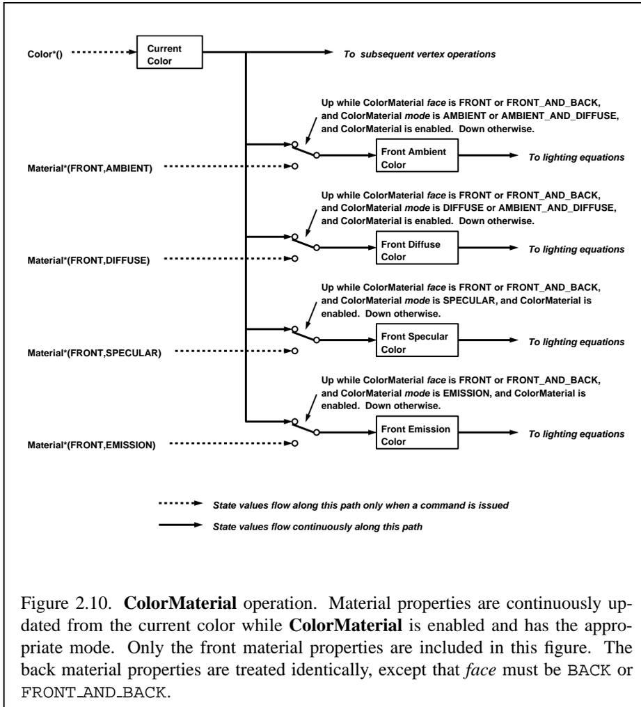
Figure 2.10. **ColorMaterial** operation. Material properties are continuously updated from the current color while **ColorMaterial** is enabled and has the appropriate mode. Only the front material properties are included in this figure. The back material properties are treated identically, except that *face* must be BACK or FRONT\_AND\_BACK.
