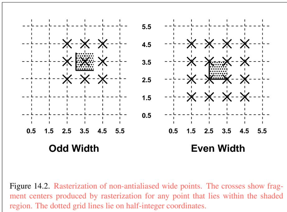
Figure 14.2. Rasterization of non-antialiased wide points. The crosses show fragment centers produced by rasterization for any point that lies within the shaded region. The dotted grid lines lie on half-integer coordinates.
