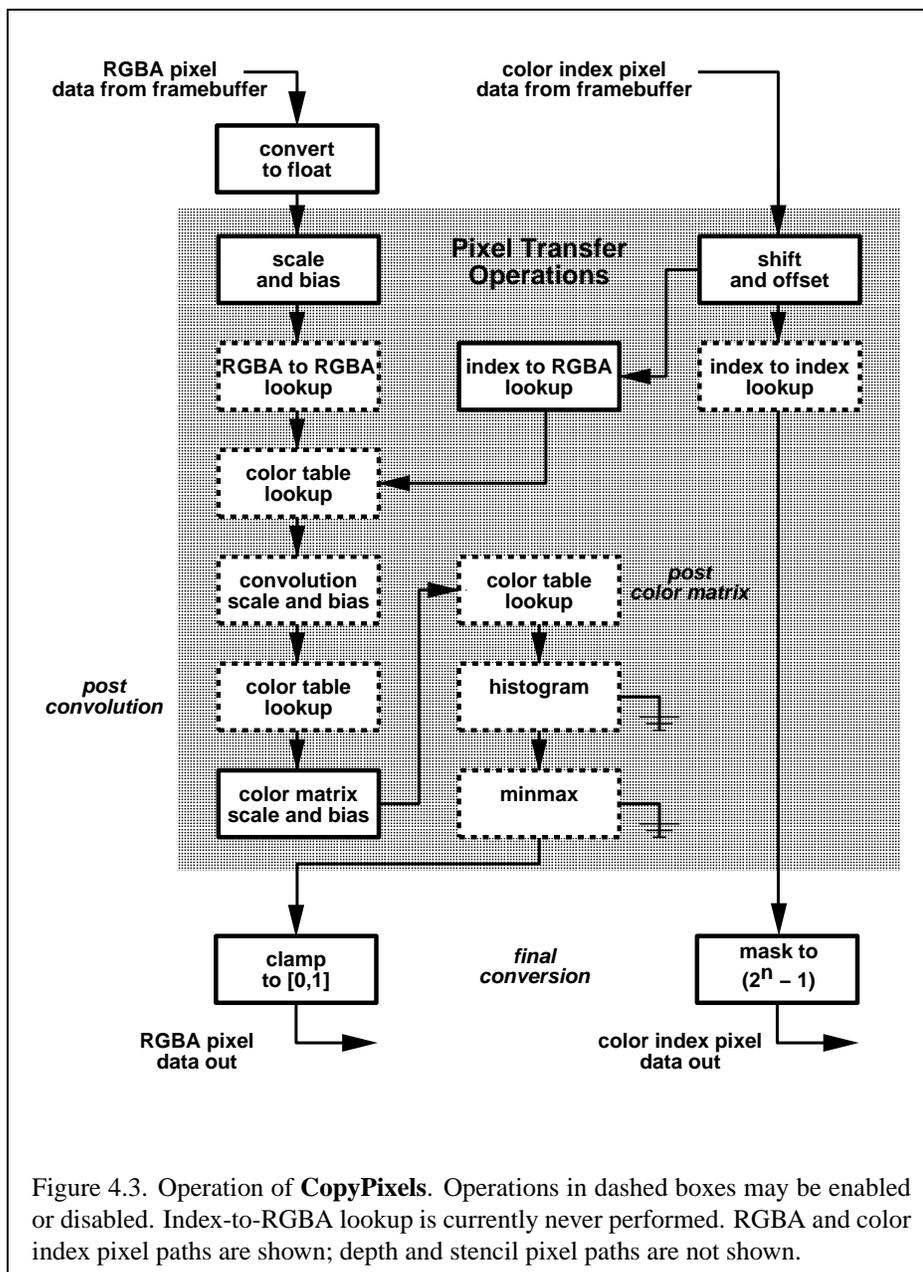
Figure 4.3. Operation of **CopyPixels**. Operations in dashed boxes may be enabled or disabled. Index-to-RGBA lookup is currently never performed. RGB and color index pixel paths are shown; depth and stencil pixel paths are not shown.
