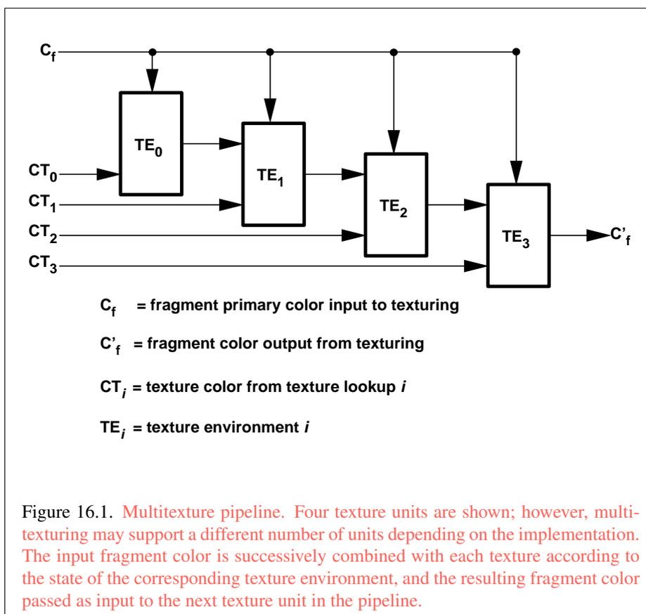
Texturing is enabled and disabled individually for each texture unit. If texturing is disabled for one of the units, then the fragment resulting from the previous unit is passed unaltered to the following unit. Individual texture units beyond those specified by `MAX_TEXTURE_UNITS` are always treated as disabled.
