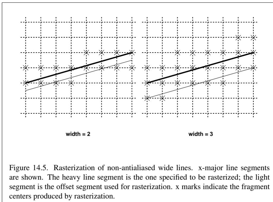
rounded to the nearest integer value, and in any event no less than 1. If rounding the specified width results in the value 0, then it is as if the value were 1.
