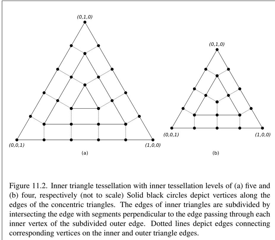
Figure 11.2. Inner triangle tessellation with inner tessellation levels of (a) five and (b) four, respectively (not to scale) Solid black circles depict vertices along the edges of the concentric triangles. The edges of inner triangles are subdivided by intersecting the edge with segments perpendicular to the edge passing through each inner vertex of the subdivided outer edge. Dotted lines depict edges connecting corresponding vertices on the inner and outer triangle edges.
