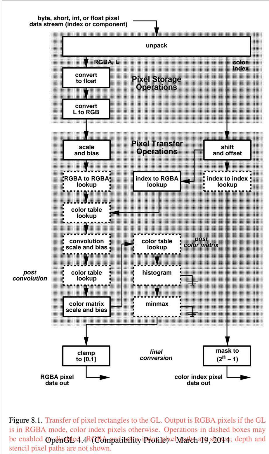
Figure 8.1. Transfer of pixel rectangles to the GL. Output is RGBA pixels if the GL is in RGBA mode, color index pixels otherwise. Operations in dashed boxes may be enabled or disabled. OpenGL 4.4 (Compatibility Profile) March 19, 2014; depth and stencil pixel paths are not shown.
