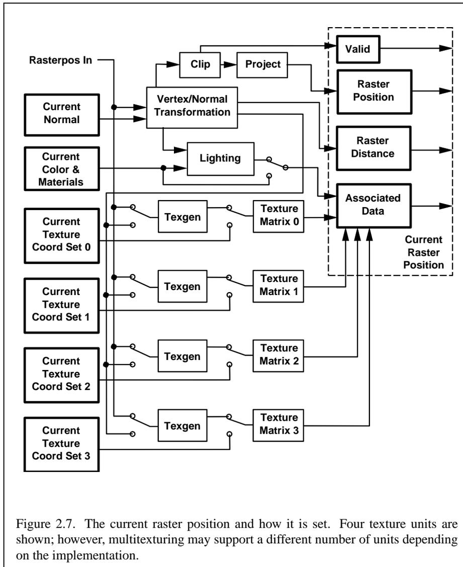
Figure 2.7. The current raster position and how it is set. Four texture units are shown; however, multitexturing may support a different number of units depending on the implementation.
