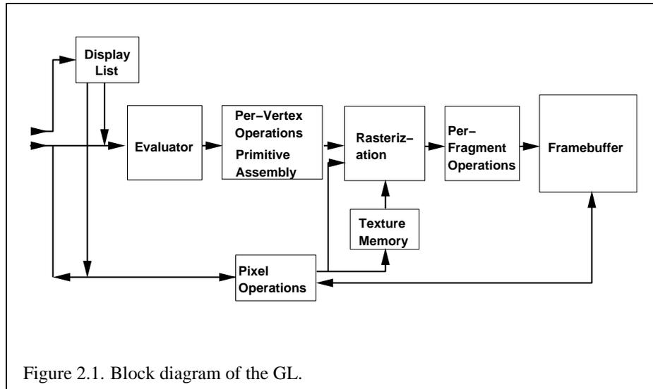
Figure 2.1. Block diagram of the GL.
