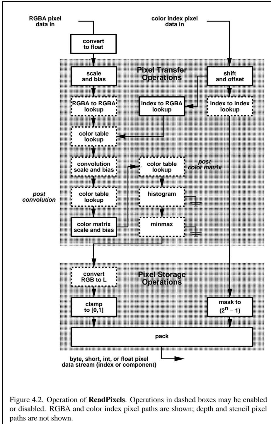
Figure 4.2. Operation of **ReadPixels**. Operations in dashed boxes may be enabled or disabled. RGBA and color index pixel paths are shown; depth and stencil pixel paths are not shown.
